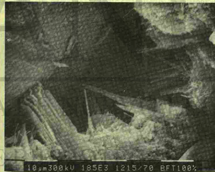
Fig. 7. SEM micrograph of normal 100% type 10 cement-concrete [Magnification x 1850], shows Ca(OH) 2 platelets and CSH fibres bonding well with coarse aggregates after 28-days of curing.
