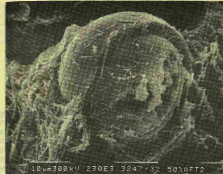
Fig. 16. SEM micrograph of high flyash concrete (50%flyash + 10%CSF), reveals a partly reacted flyash particle with its envelope broken and with needle-like crystals of ettringite scattered around, after 300 freezing and thawing cycles [Magnification x 2300].
