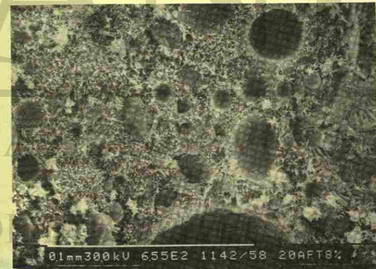
Fig. 17. SEM micrograph of 20% flyash + 10% CSF air-entrained concrete reveals a matrix with numerous air-void sockets filled with needle-like crystals, after 300 freezing and thawing cycles [Magnification x 655].
