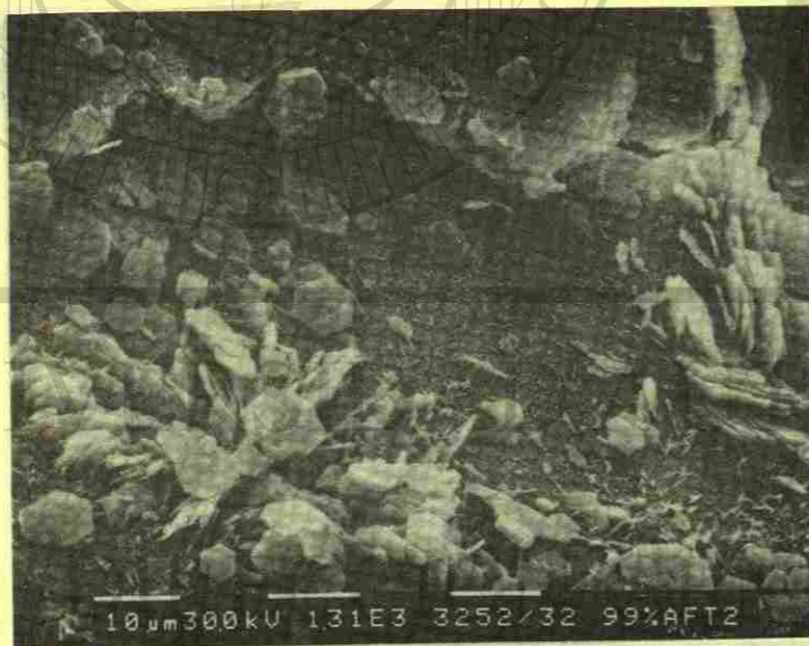
Fig. 15. SEM micrograph showing cracked matrix of normal concrete with platelets of \text{Ca(OH)}_2 crystallised over hydration products in cracks, after freezing and thawing cycles [Magnification x 1310]. Some needle-like ettringite crystals are also observed.
