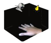
Figure 5.1 – Background, camera, and illumination arrangement.
