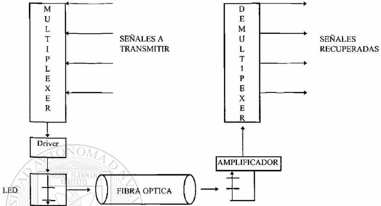
Fig. 9.4 Sistema Multiplexor / Demultiplexor.
